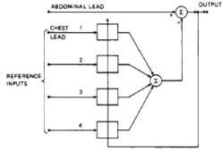
Fig. from Adaptive Signal Processing, Widrow, Stearn Fig. 15. Multiple-reference noise canceller used in fetal ECG experiment.
